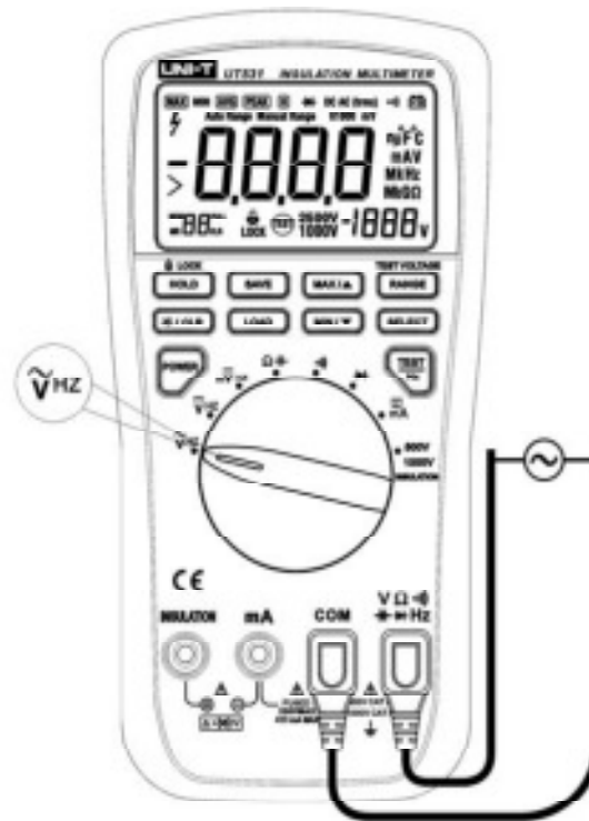
Figure 5. Measuring AC Voltage
